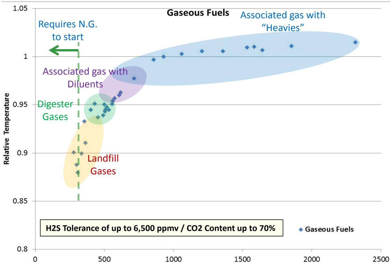
Fuel Lower Heating Value (Btu/ft3); dry basis at 14.7 psi (101 kPa) and 59F (15C)
